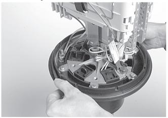
3.12.1 Place the O-ring back on a clean base ! Remove the silica-gel from the bag and place it in the closure.
