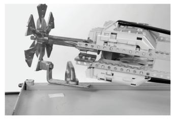
3.2.1 Install the cable attachment plate holder (FIST-GCOG-CAPH) to the cable attachment plate and use the clamp to mount it on a table.
