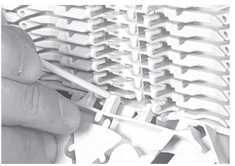
3.9.6 To remove the tray put the fiber guiding pin between the lip on the wraparound groove plate and the tray, and move laterally towards \$1.
