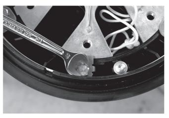
3.7.3 Slide and position the base over the gel block and tighten the securing screws of the cable attachment plate.
