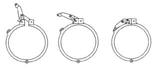
3.12.3 Install the dome and close it with the clamp.
