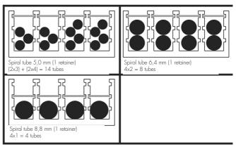
3.10.2 Tube holder capacity Number x outer diameter loose tube (mm)
