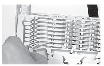
3.9.9 Pull gently on the fibers in the tray and make sure that the fibers are well contained in the routing block and wraparound groove plate.
