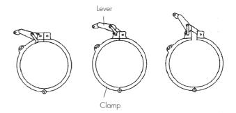
3.1.1 Open and remove the clamp
