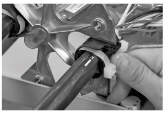
3.6.4 Slide the base over the cables and position the cable retention devices in the cable attachment plate.
