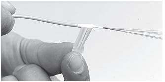
3.8.4 Clean and degrease the fibers and wind some PTFE tape around the transition from tube to fibers for protection.
