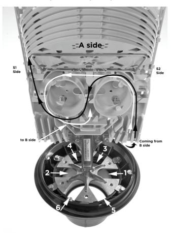
3.9.1 Fibers can be routed between As1, As2, Bs1 and Bs2. In case fibers have to be routed from side A to side B, use the window. Select the cable termination in such a way that a minimum of fibers will cross and have to be routed through the window. Therefore the selection of ports according to the cable lay-out is important.
