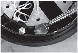
3.7.8 Remove the cable attachment plate holder and place the base in the pole/wall mounting bracket for ease of working. Tighten all the securing screws of the cable attachment plate.
