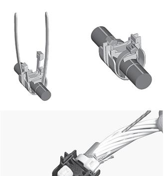
3.6.3 Heat the cable jacket and position the cable retention device 5 mm behind the cable jacket end. Push the cover in the cable retention device and make sure that the teeth of the device and the cover are pressed in the cable jacket. Tighten the tie wraps (with the tie wrap tool).
