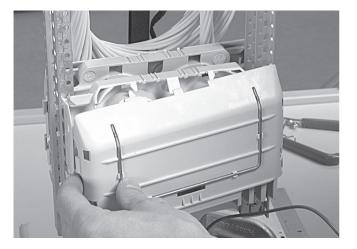
3.9.2 Remove the hook and loop fastener and routing block cap. To remove the routing block cap lift the two snaps at one side of the routing block cap.
