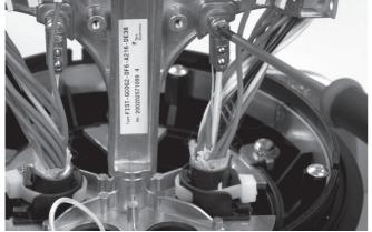
3.7.6 Mount the UCT (strength member fixation) on the strength member (if needed cut the strength member to length). Fix the eyelet on the closure bracket.
