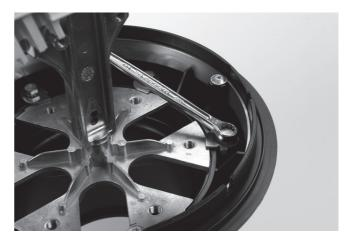
3.1.3 Loosen the securing screws of the cable attachment plate and take out the cable attachment plate with the pre-installed UMS.
