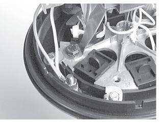
3.11.1 In case of grounding, mount the grounding wire on the grounding bolt.
