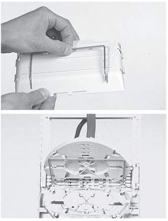
3.9.7 Identify the tray to be worked on and make it accessible. If the routing block and trays are in vertical position, you will have to support the trays above the selected one using the tray wedge which fits in the holes of the wraparound groove plate. Position the wedge carefully such that the groove is still accessible for the fibers and be careful not to push the wedge against fibers.
