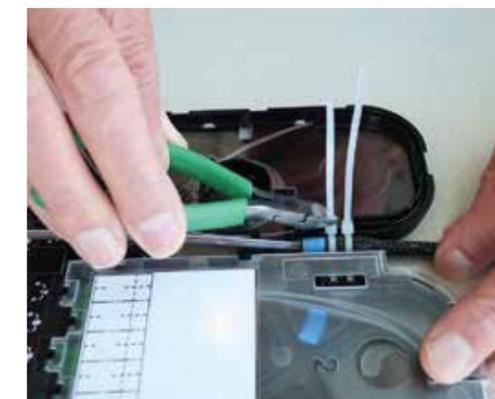
**5** **Remove the splice wheel from the cassette.** Lift the splice wheel from the cassette, unwind the inner fiber ribbon (counterclockwise), and extend the splice wheel and ribbon out beyond the front of the cassette. Remove fiber from splice cassette.
