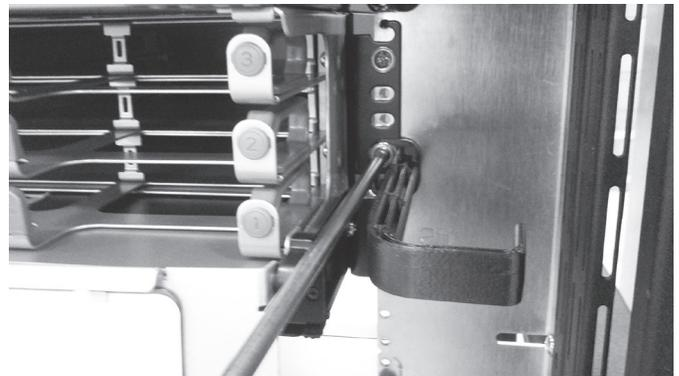
(3.) Connect Fiber Patch cords to module and run the cables out of chassis and over the accessory kit Vertical Cable Guide. Do this for both sides of the chassis.
