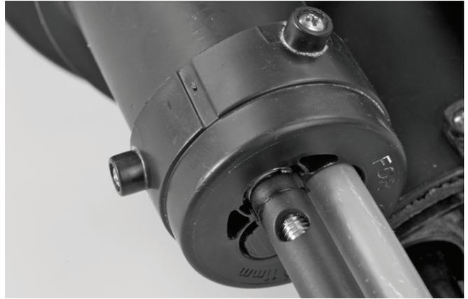
3.5.7 Tighten the trigger till it butts up with the flange. In case of 2 out when only 1 cable is installed, use the dummy rod.
