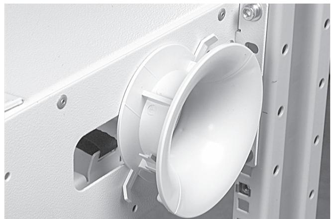
2.4 A horn is needed at the side where the pigtails are entering the shelf. Install the horn by positioning it centrally in the opening at the side of the shelf. Align the small knobs with the slots in the side, pull back the two locking lips of the horn and turn until the locking pins click into both positioning holes.
