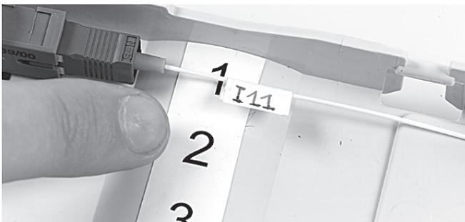
3.2 The identification (printed on the flags next to the connector boot) of the pre-assembled 900 micron pigtails is as follows
