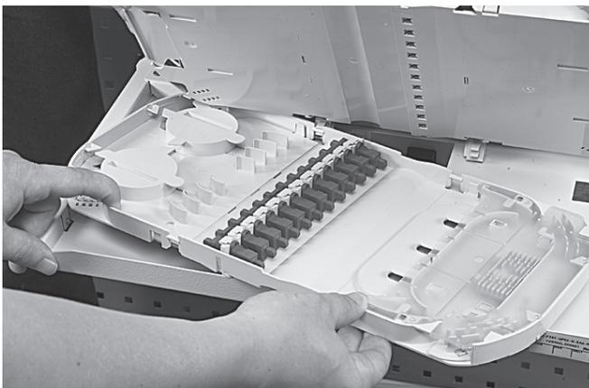
2.1 When necessary, one can remove the appropriate tray by pulling it out of the hinge.
