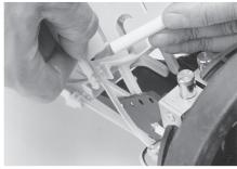
8.3 Use tray wedge to keep the tray in upward position.
