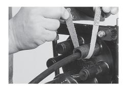
11.8 Place cable seal over the drop outlet of FOSC base. When cable seal butts against the base, mark the sleeve length on cable sheath.
