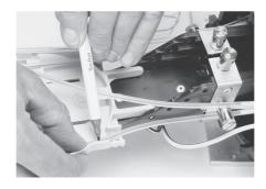
7.1.2 Carefully cut the transportation tubes at the mark and secure to splice tray with two tie wraps. The transportation tube may not be in contact with fibers stored in the organizer. Other tubes should be laid out of the way of the bottom tray. Alternatively, additional trays may be installed to store the fibers (see section 9). Cut the transportation tubes in the organiser/tray. Always place transparent cover over tray.
