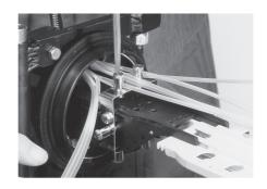
5.6 If required, connect shield continuity wire of both cables with shield continuity clip. Talk pairs, if present, will be connected together according to the local procedures.
