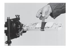
9.2 Ensure seal areas and sealing ring are clean and sealing ring is in place at the base.
