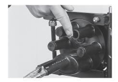
11.2 Remove any dirt, mud or other contaminants from the cable sheath for approximately 2 meters with a clean cloth. Take the cable seal sleeve from the kit FOSC-B/D-CSEAL1-NT and slide it over the cable. The non-coated edge of the sleeve and the arrows should be pointed to the base of the closure.
