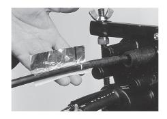
11.10 Slide the cable seal over the port.
