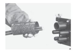
4.4 Slide the cables through the opened oval port. Prepare cables as described in section 5 (cable preparation).
