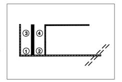
7.2.2 After each splice is made, the splice should be stored as indicated on the drawing (see 7.2.1.). First protector in position 1, the second in position 2. Continue for other fibers. Fiber n°5 will be in position 1 of next location. Coil the excess length of fiber each time you have positioned the splice protector.
