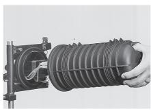
10.3 Remove gently the sealing ring. Keep the sealing ring and seal area of the closure free of dirt (if needed rinse with clear water).
