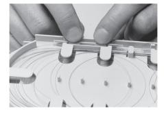
7.1.7 Upon completion of splicing, install the clear protective cover on the tray. Secure cover by installing the hook and loop fastener strip around the trays and cover.
