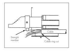
5.5 Slide strength members into clamps and tighten. Cut away the excess length of strength member.
