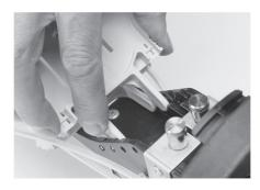
8.2 Proceed for fiber splicing as described from point 7. However, provide enough slack on transportation tube such that no severe bending or kinking of tube may occur during hinging.
