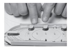
7.1.6 For 12 fiber capacity tray, two fusion protection sleeves should be installed on top of one another in one splice holder.
