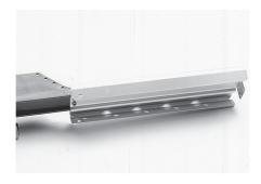
15.3 Attach the slack tray with the nuts and bolts. Tighten the nuts. Re-install the bottom tray by aligning the tray pins with the bottom holes of the bracket. Squeeze tray pins and slip tray into the bracket
