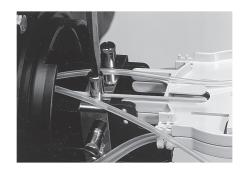
11.6 Thoroughly clean port and cable sheath with the cleaning tissue over a distance of 100 mm from the edge of the port.
