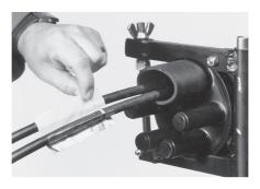
6.5 Slide the oval cable seal over the oval port. Install the branch-off clip. Check that the heat-shrinkable sleeve butts up against the FOSC-base and the branch-off clip is completely inserted. Tape the two cables together.
