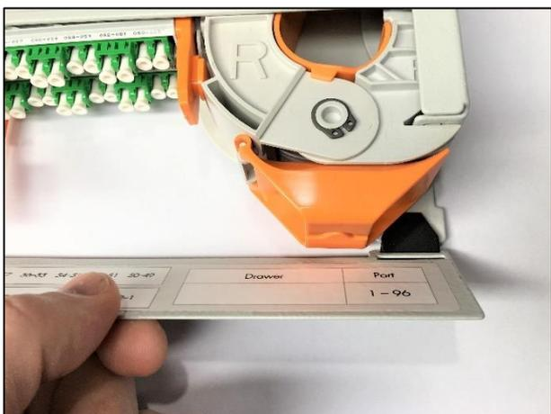
10.1.3 Take the front cover, place it into the slot of the hinges under an angle of 45°, push until the cover is fixed. Repeat on the other side.
