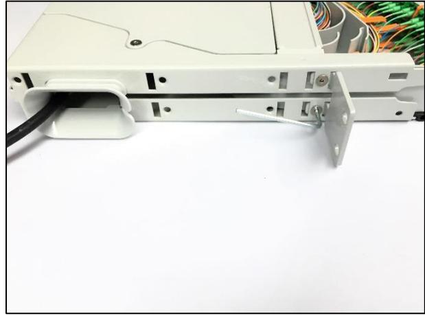
10.2.1 Select the preferred mounting position. Mount the bracket with the 2 small provided screws. Open the shelf for gaining space to mount the left and or right side.
