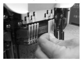
10.7 Horizontally place the Fig.8 cable and use cable tie to fix the cable as shown.
