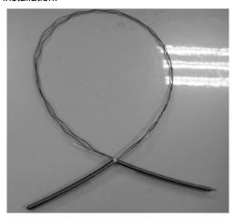
5.2 Clean the cable sheath, where it contacts gel, with cleaning tissue provided.
