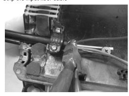
6.4 Degrease the fiber bundle and slide the transportation tubes over the fibers with overlap 50mm
