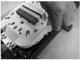
4.3 Unscrew the upper clamps where you will install the cable.
