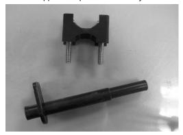
4.5 Separate the dummy rod and the blocking ring, as shown
