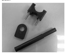
4.6 According to the cable range choose the appropriate side of the cable clamp and remove the white sleeve layer installed on the lower clamp if necessary (refer to Table 1).
