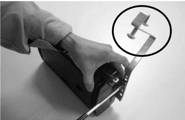
5.2 Secure the closure onto the strand wire firmly.
