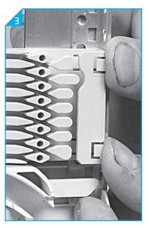
8.1.2.1 Secure the wraparound grooveplate on the UMS profile by putting the plate with the long protrusions in the S1 UMS-profile and sliding the plate in the S2 UMS-profile until it snaps.
