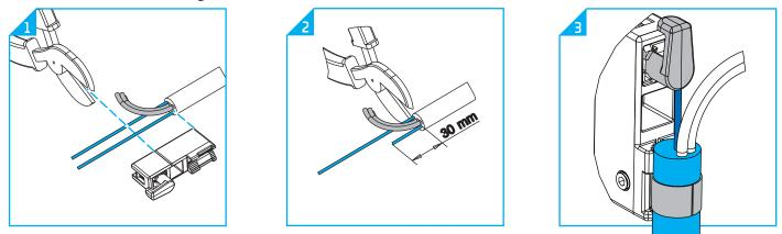
9.3.2.1 Cut one of the two strength members to a length of 30 mm. To mark this distance, the line on the side of the CTU can be used. Hold the cable jacket flush with the bottom of the CTU and mark the strength member at the height of the line
