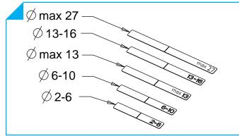
Measure the cable diameter to select the correct CTU and/or the correct cable retention metal strap.
