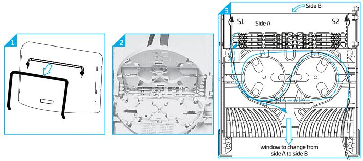
14.1 Remove the hook and loop fastener and the FAS cover to make the FAS accessible. If the routing block and the trays are in vertical position, the trays above the selected tray or FAS should be supported by the wedge to provide access to the selected tray/or FAS. The wedge is located on top the FAS cover. Pull on the wedge to detach the wedge from the FAS cover.
