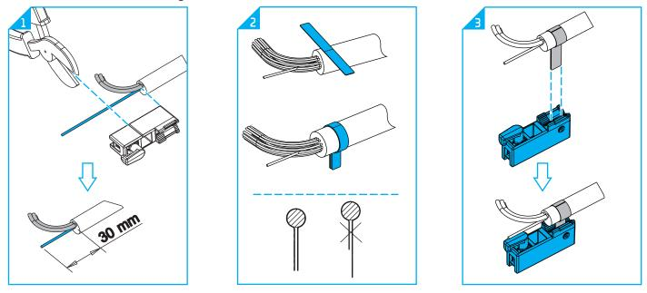
9.3.1.1 Cut the strength member to a length of 30 mm. To mark this distance, the line on the side of the CTU can be used. Hold the cable jacket flush with the bottom of the CTU and mark the strength member at the height of the line.
