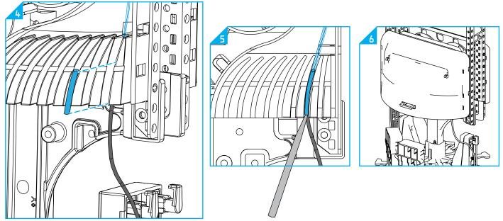
13.4 Insert the tube/subunit (with the Teflon tape) in one of the channels in the FAS block. Press the piece of silicone orange tubing in the channel on top of the tube/subunit. **Note**: Position the tube/subunits in a logical order, avoid making crosses underneath the FAS block. **Note:** place the end of the orange tube/subunit at the start of the channel. This makes it easier to remove the silicone orange tubing.
