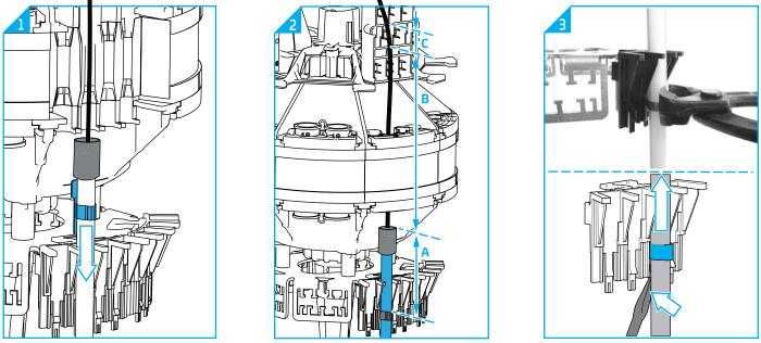
15.3.1 Install the gas/water blocking device per local practice on the micro duct cable transition. Make sure the width of the device fits in the required configuration. Position the cable in the gel port, and slide the crimp ring in the receiver. Make sure the gas/water blocking device is properly positioned between the gel seal segment and the receiver.
