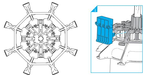
8.2.2.1 Select the assigned port in the starbracket and slide the two slots of the CTU holder over the flanges of that port on the star bracket.
