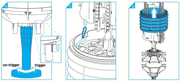
7.4 To remove the base, the trigger system should be un-triggered. The bottom of the seal block will move down over the studs. When the base is flush with the end of the ribs on the studs, the gel is fully uncompressed and the base can be removed.
