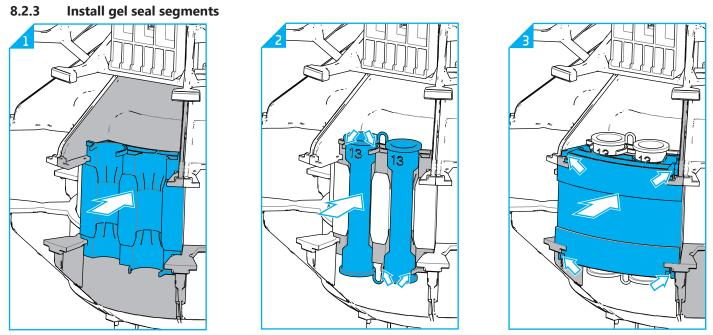
8.2.3.1 To install the gel segments the trigger system should be un-triggered state. Slide the inner gel segment over the 4 ribs of the seal block.
