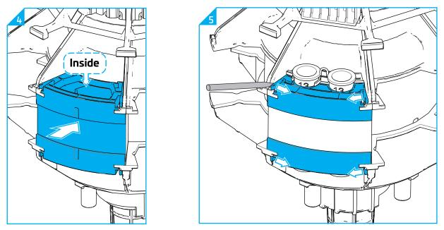
8.2.4 To install a **SKG-DUMMY**, slide the dummy gel seal (one piece) over the 4 ribs until it snaps. Verify the proper orientation of the dummy gel seal, see image above.
