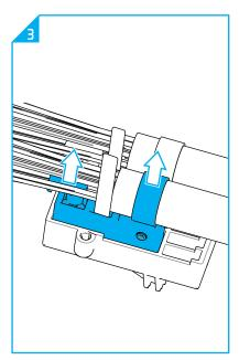
10.2.1 CTU installed in the CTU holder. The 2 snap hooks in the CTU cavity prevent the CTU from being removed.
