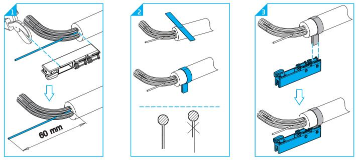
9.3.5.1 Cut the strength member to a length of 60 mm. To mark this distance, the line on the side of the CTU can be used. Hold the cable jacket flush with the bottom of the CTU and mark the strength member at the height of the line.
