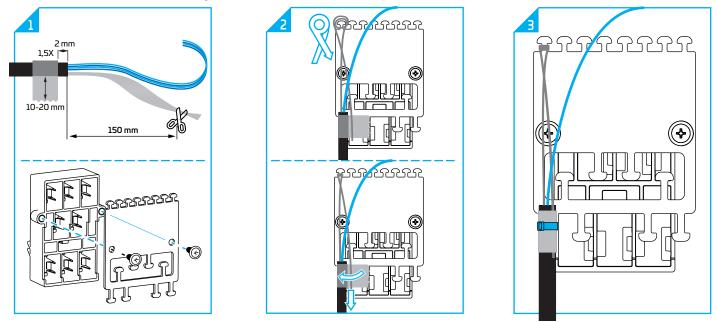
9.4.1.1 Cut the aramid yarn to a length of 150mm. Apply 1,5 turn of felt tape around the cable and keep 10 to 20 mm over length. Secure the metal plate onto the CTU holder with the two ejot screws.
