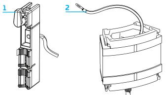
To ground, bond and/or tone cables two kits are applicable: the SKG-FDTHR (feed through) and the CTU-G-GRND (CTU-grounding).
