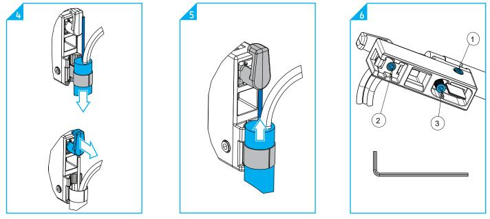
9.3.1.4 To insert the strength member in the strength member holder, first pull the cable slightly back (making sure the jacket doesn't pass the metal strap), then move the strength member holder forward.
