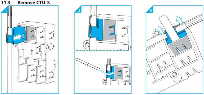
11.3.1 CTU installed in the CTU holder. The snap hook in the CTU cavity prevent the CTU from being removed
