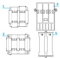
An SKG (except SKG-DUMMY and SKG-FDTHR) always contains: a CTU holder, dummy plugs and two pieces of gel seal segments (figure showing example of an SKG2 kit).
