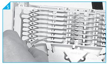
14.4 Route the fiber in the correct groove of the wraparound grooveplate to the entrance of the identified tray. Fiber must be routed in the groove behind the hinge of the tray!
