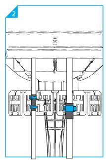
12.2.1 Mount the external cable bracket with the 4 screws onto the base using a Phillips screwdriver. (Preferable before the cables are installed.)
