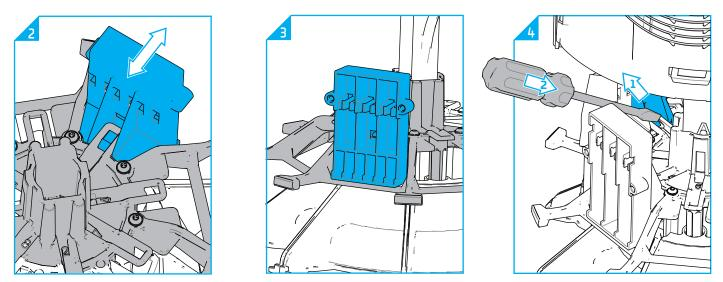
8.2.2.2 The snaphook on the CTU holder will fall into the opening in the bracket. The CTU holder can float to be able to position itself towards the position of the strength member.
