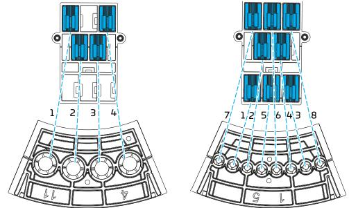
11.2.1 If installing a cable in a 4-out seal port, the position of the cable in the seal port determines the position of the CTU in the CTU holder. Observe image above.
