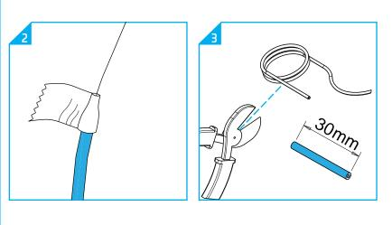
13.1 Select the tubes/subunit with the fibers to be spliced. Position the tube/subunit on top of the channel and mark the tube/subunit at the point indicated with the lines. Strip the tube/subunit between (shaving) or until the mark(s). Degrease and clean the fibers.
