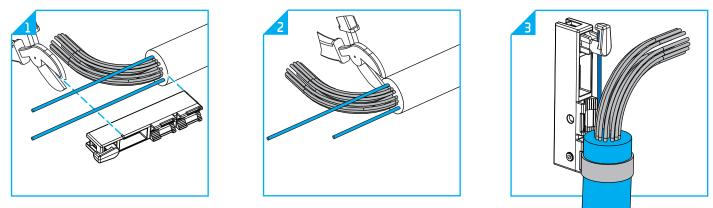
9.3.6.1 Cut one of the two strength members to a length of 60 mm. To mark the distance, the line on the side of the CTU can be used.
