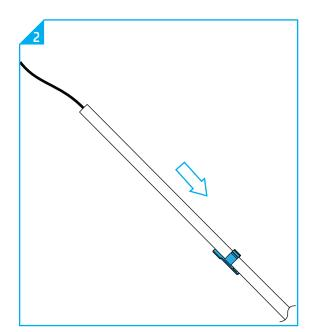
15.2.1 Install the crimp ring receiver on the external bracket. First bring the receiver through the dove tail opening, then slide the receiver downwards until a clicking sound is observed.
