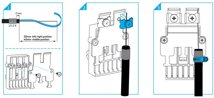
9.4.2.1 Cut the rigid strength member to length, depending on its position on the metal plate. Apply 1.5-2 turns of felt tape around the cable. Secure the metal plate onto the CTU holder with the two ejot screws.
