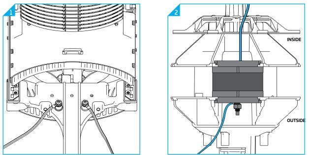
16.3.1 Attach the pre-installed wire to the tower with the bolt and the star washer mounted on a stud. More than one wire can be attached to one stud.
