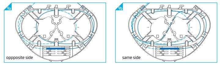
14.9 Make fusion splice per standard practice and store the splice protector centered in the splice protector holder. **Note**: The drums on the tray (islands) can be used to make a crossing/loopback on the tray. If the fibers need to be spliced enter the tray from the same side, one fiber must make an S-shaped loopback on the tray using the openings between the islands (see full line in the image above).
