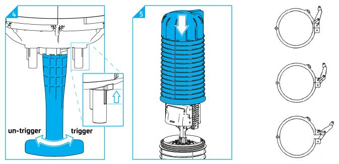
17.4 Activate the seal mechanism by turning the handle (trigger). If the second rib on the studs appears, then the seal system is properly activated.
