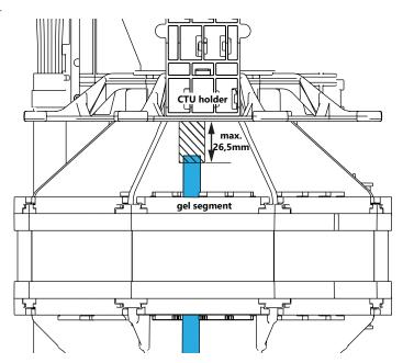
15.4.1 When selecting and installing the gas/water blocking on the micro ducts inside the closure, dimensions above need to be respected. Also verify if the width of the device fits in the required configuration. If the device doesn't fit inside the closure, install the gas blocking outside the closure.
