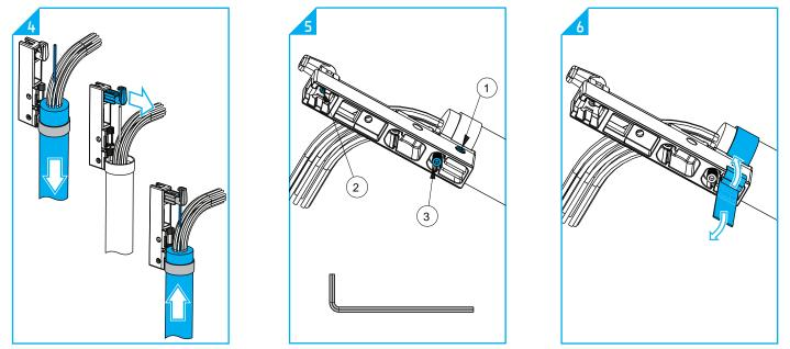
9.3.5.4 Insert the strength member in the strength member holder. First pull the cable slightly back (making sure the jacket doesn't pass the metal strap), then move the strength member holder forward and then push the cable upwards again until the central strength member butts against the strength member holders top surface. **Note**: Some strength members may need to be trimmed in width to fit properly.
