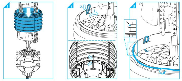
17.1 Slide the base over the fiber management system until it is in the end position.
