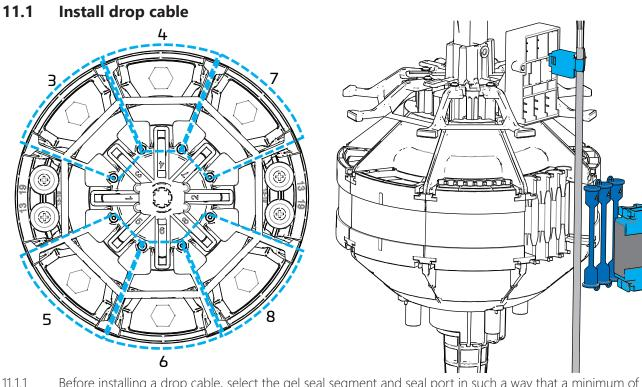
11.1.1 Before installing a drop cable, select the gel seal segment and seal port in such a way that a minimum of fibers will cross under and in the FAS block area. Drop cables can be installed in port 3,4,5,6,7 an 8.
