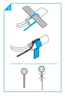
9.3.4.1 Cut the aramid yarn to a length of 80 mm.
