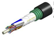
Fiber indoor/outdoor cable, loose tube gel-filled CST, 48 fiber, Singlemode G.652.D and G.657.Al, Meters jacket marking, Black jacket color
