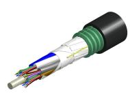
Fiber OSP cable, PE, Stranded Loose Tube Gel-filled CST, 72 fiber, Multimode OM4, Meters jacket marking, Black jacket color
