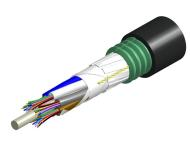
Fiber OSP cable, PE, Stranded Loose Tube Gel-filled CST, 48 fiber, Multimode OM4, Meters jacket marking, Black jacket color
