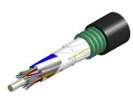
Fiber OSP cable, PE, Loose Tube Gel-filled CST, 48 fiber, Singlemode G. 652.D and G.657.A1, Meters jacket marking, Black jacket color
