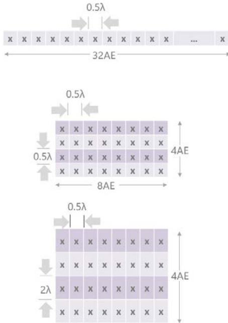
Figure 37: 64T64R mMIMO panel configuration
