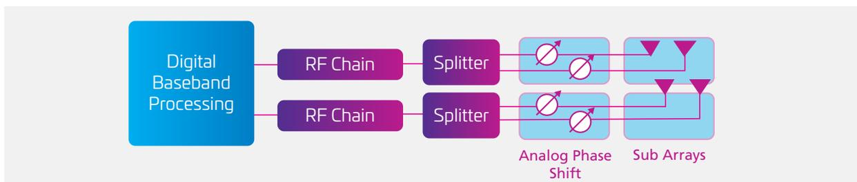
Figure 18: Hybrid beamforming
