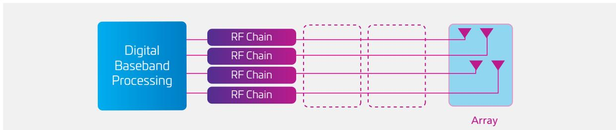
Figure 17: Digital beamforming
