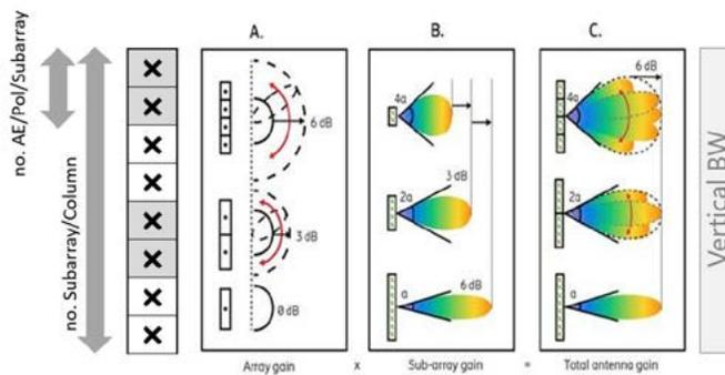
Figure 12: Subarrays gain, modified from [8]
