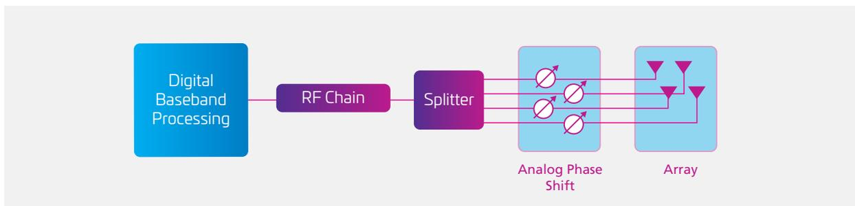
Figure 16: Analog beamforming
