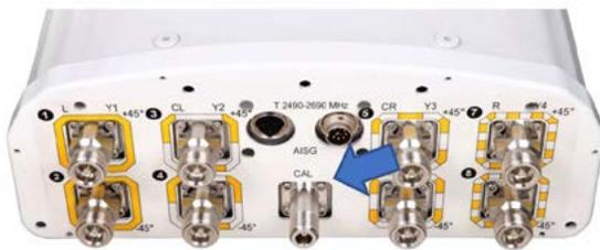
Figure 27: Calibration port on a CommScope antenna
