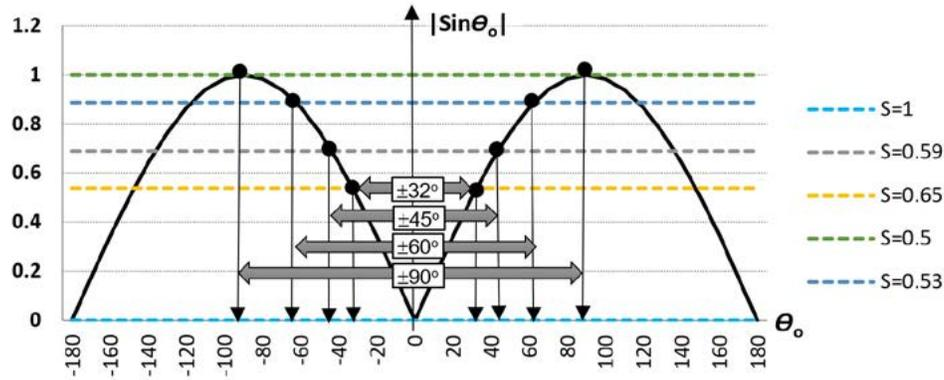
Figure 21: Column spacing vs. max scan angle
