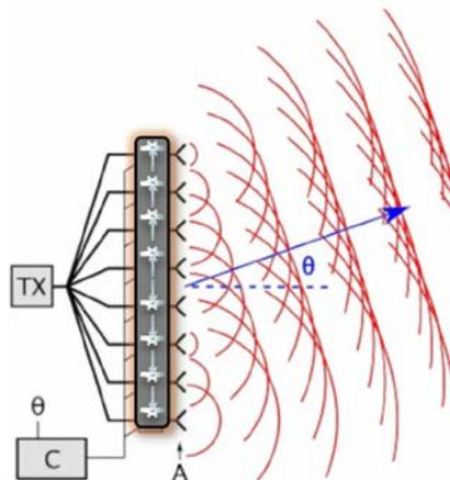
Figure 14: Effect of phase shift
