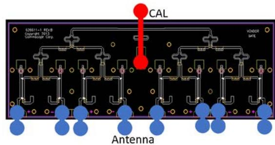
Figure 28: Calibration board
