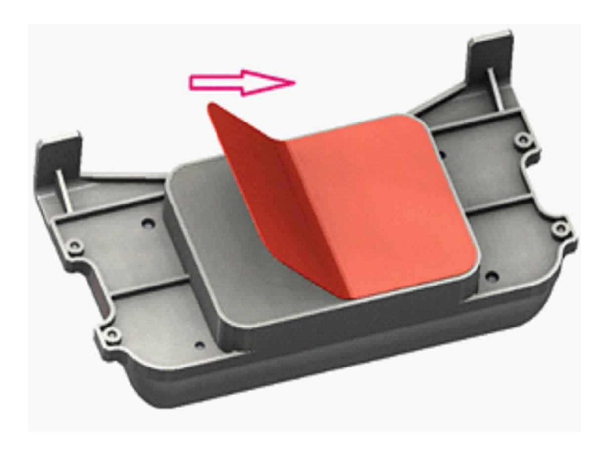
2 Put down the support vertically until the adhesive tape stick on the top cap of antenna.
