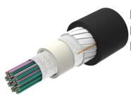
Fiber OSP cable, Non-Armored, All-Dielectric, Arid-Core, Dry Central Tube Rollable Ribbon, 432 fiber, Singlemode G.652.D and G.657.A1, Gel-free, Feet jacket marking, Black jacket color
