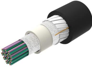
Fiber indoor/outdoor cable, All-Dielectric, LSZH Riser-Rated, Gel-Free, Central Tube Rollable Ribbon, 288 fiber, Singlemode G.652.D and G.657.A1, Feet jacket marking, Black jacket color, Cca flame rating
