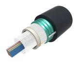
Fiber OSP cable, Steel Armored, Arid-Core, Dry Central Tube Ribbon, 24 fiber, Singlemode G.652.D and G.657.A1, Feet jacket marking, Black jacket color
