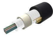
Fiber indoor/outdoor Cable, LSZH Riser All-Dielectric Central Tube Ribbon, Singlemode G.652.D and G.657.A1, 24-fiber, feet jacket marking, black jacket color
