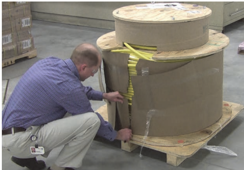
Figure 4. Cutting Off Cardboard Wrap on Cable Spool
