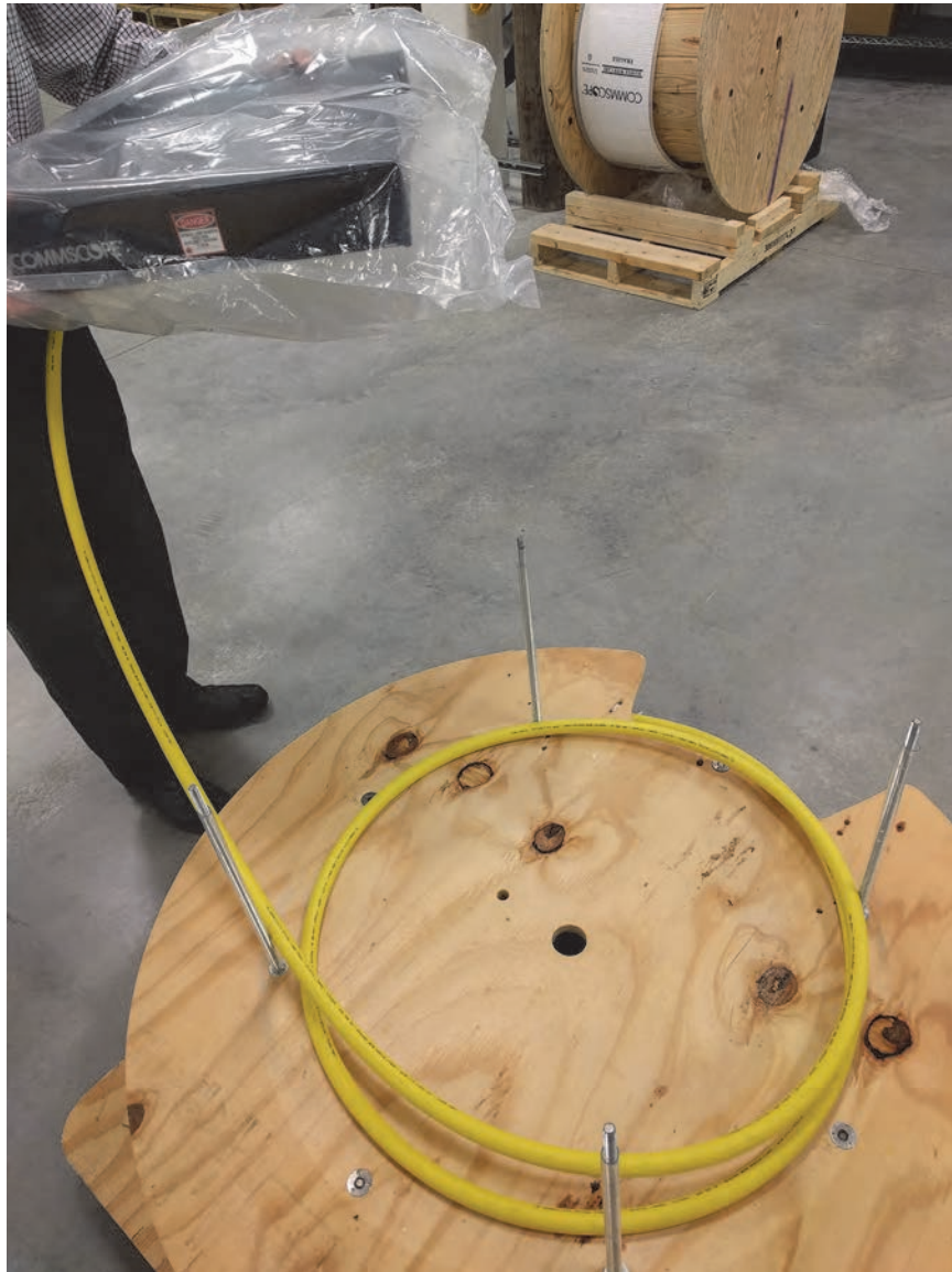
Figure 11. Lifting Off EHD Panel
