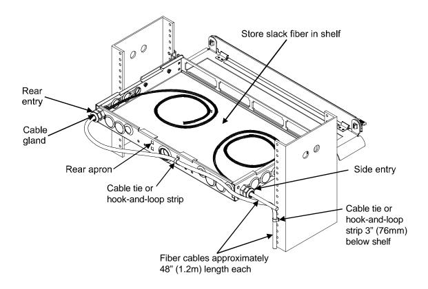
**Note:** These instructions cover only the cable gland method of securing fiber cables to the shelf.
