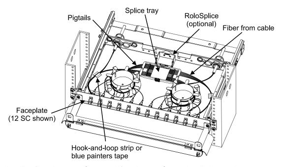
After installing fiber drums per Step 1 and faceplate per Step 2, install adapters into cutouts provided in faceplate.
