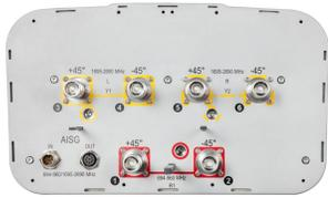
6-port sector antenna, 2x 694–960 and 4x 1695–2690 MHz, 65° HPBW, 3x RET with manual override.
