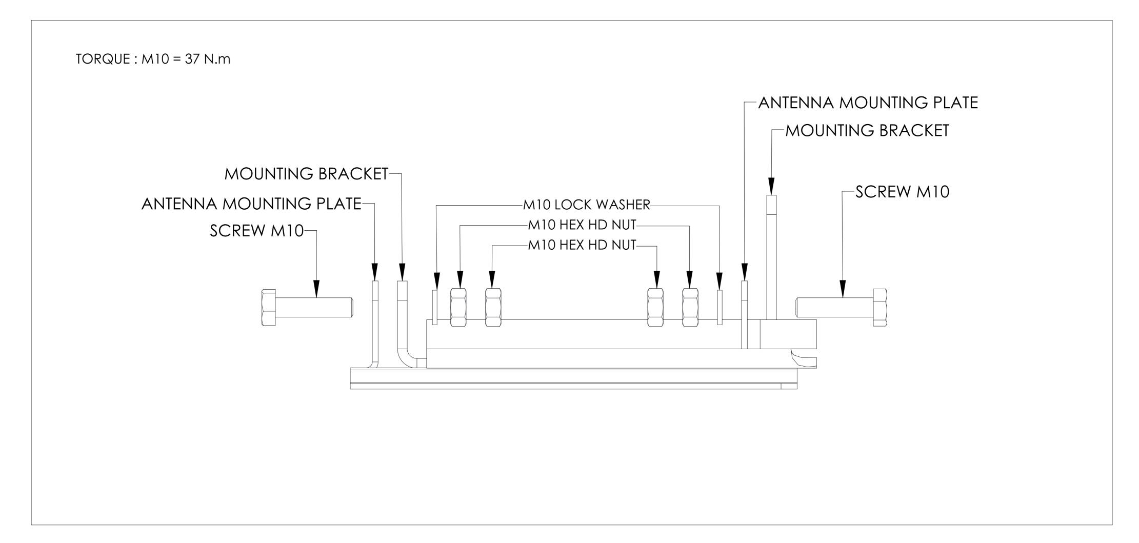
Figure 3. Attaching 627281 Mounting Bracket to Antenna.
