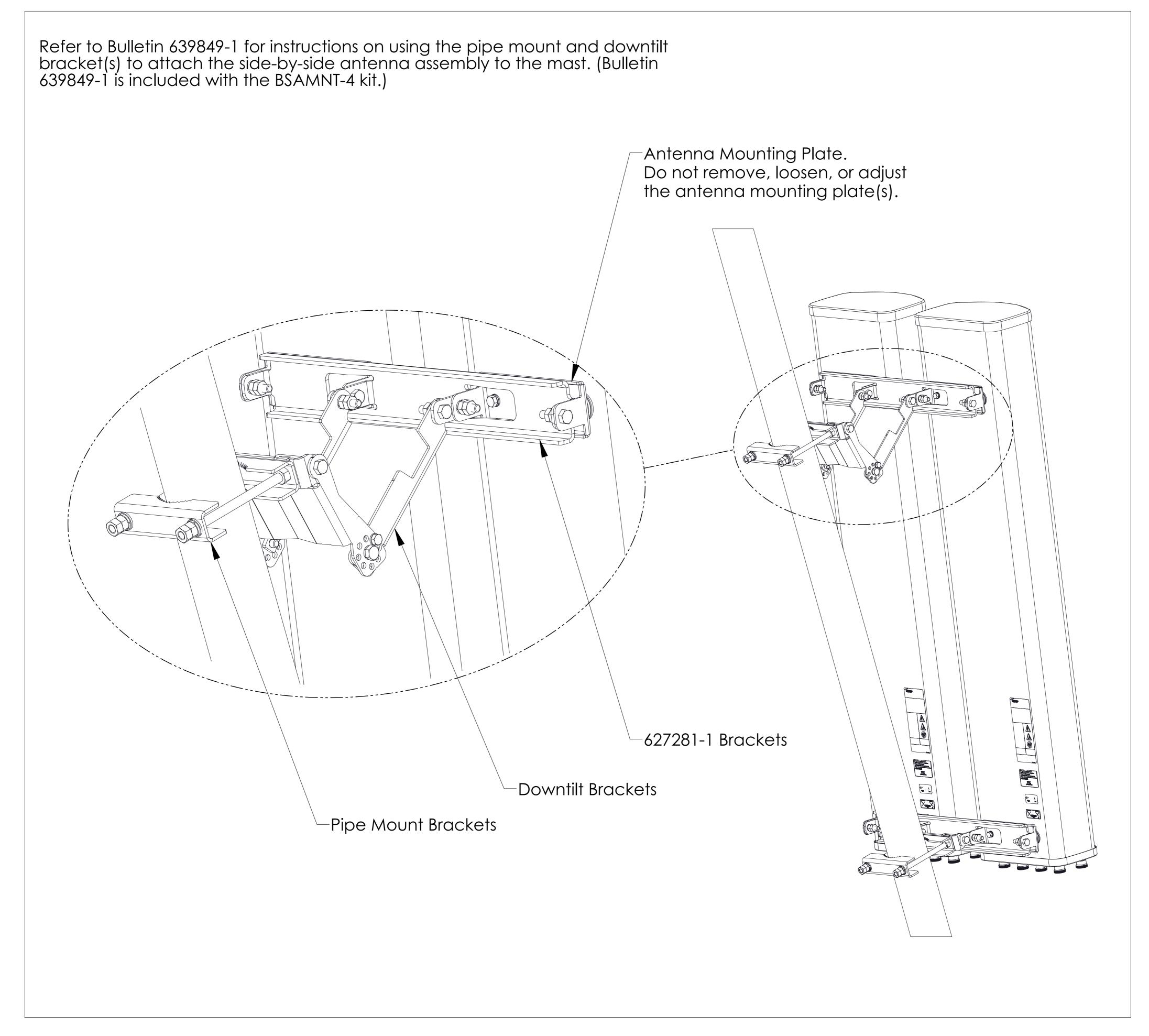
Figure 4. Antenna Assembly Attached to Mast Using BSAMNT-SBS-1-2 Mounting Kits.
