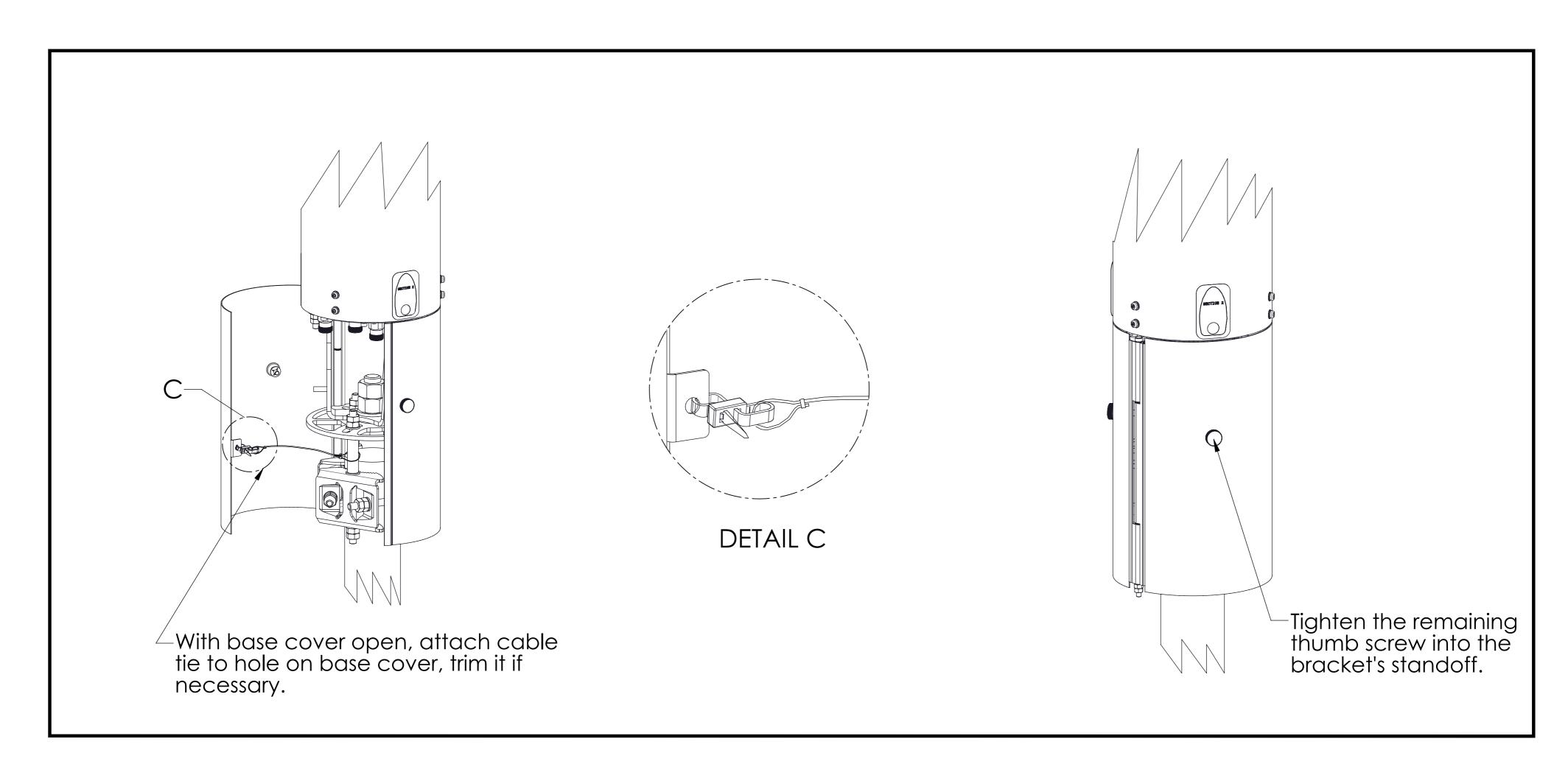
Install the lanyard on the base cover and secure the other base cover on the bracket
