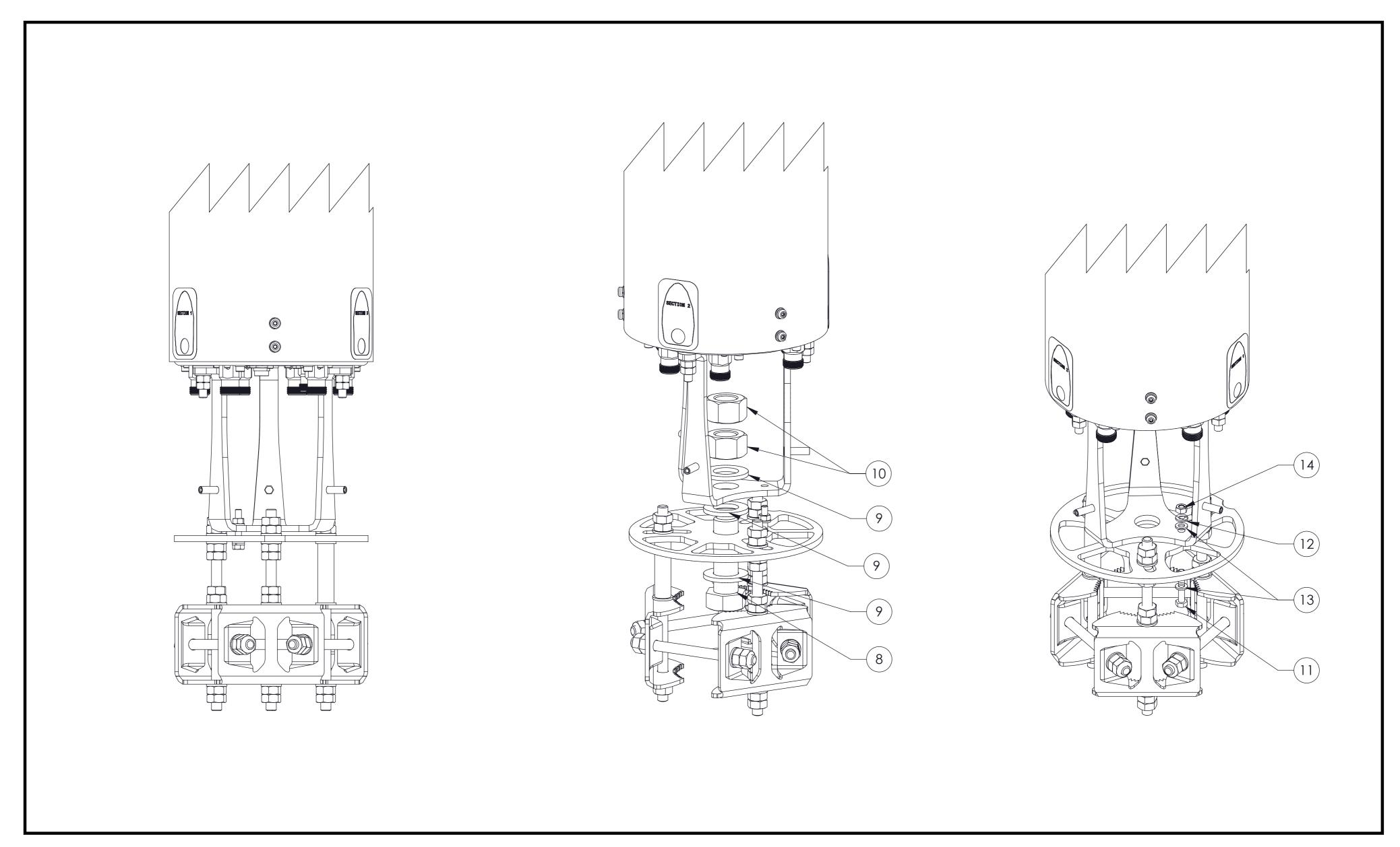
Assemble mount kit to antenna
