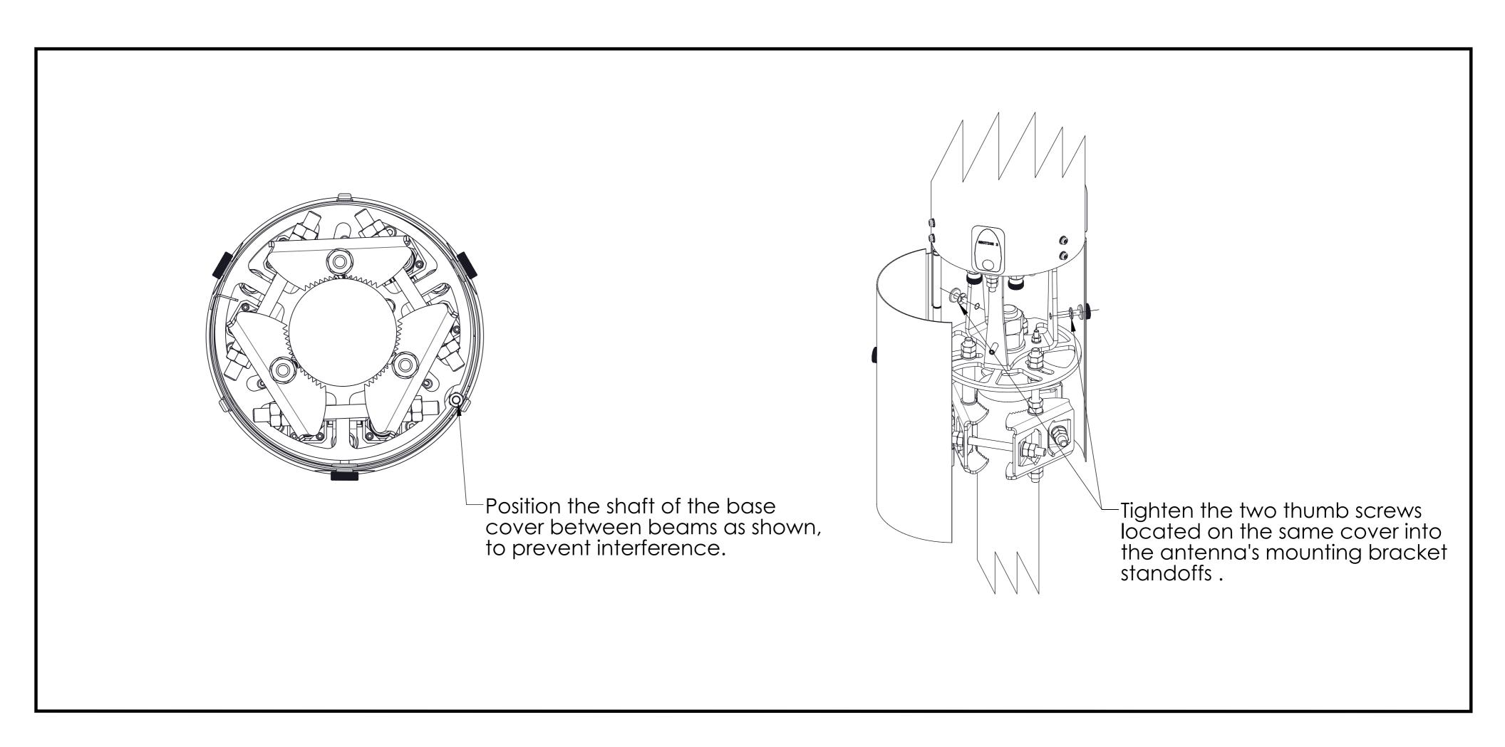
Install the base cover on the bracket
