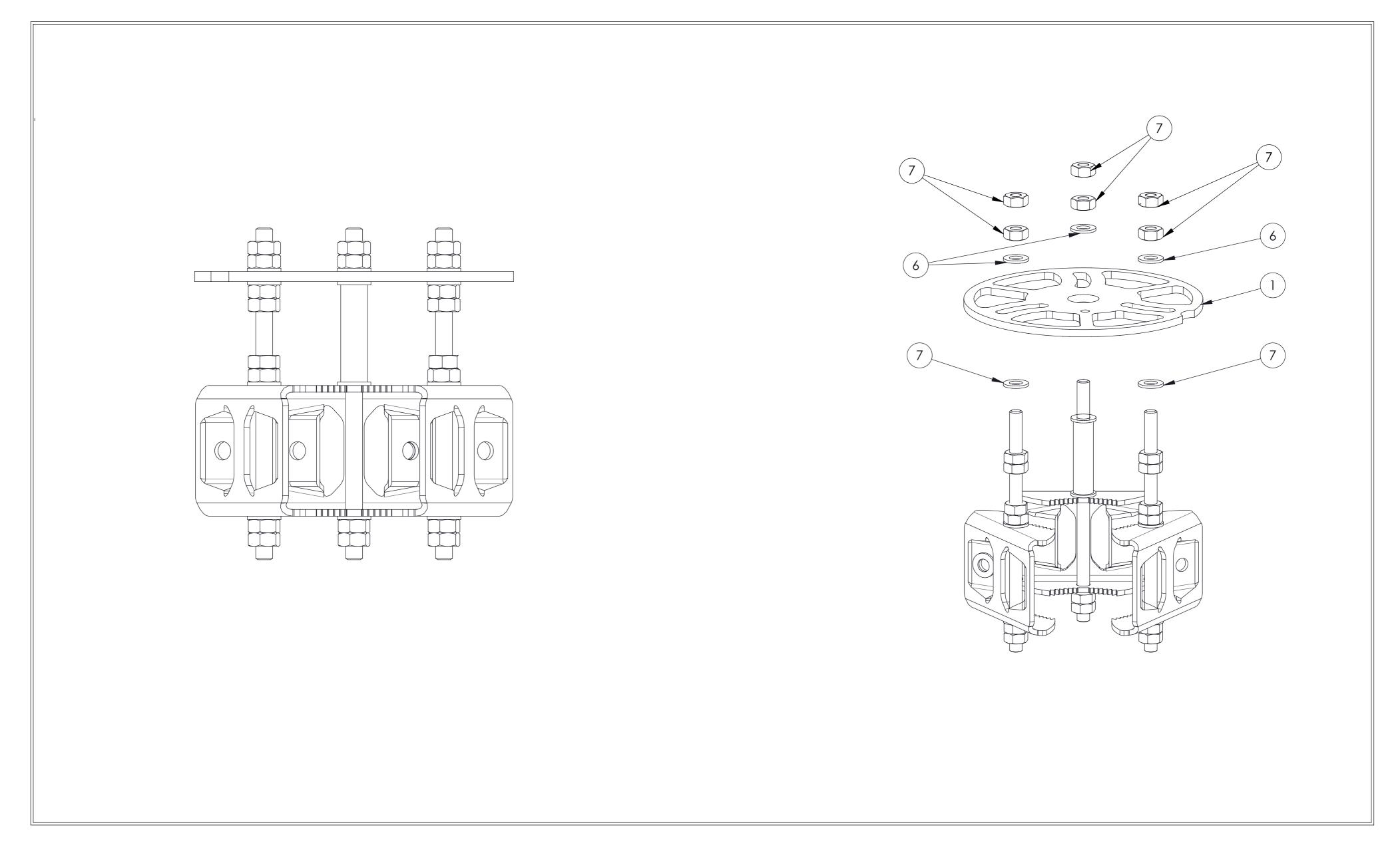
Assemble top mount bracket to pipe clamp brackets
