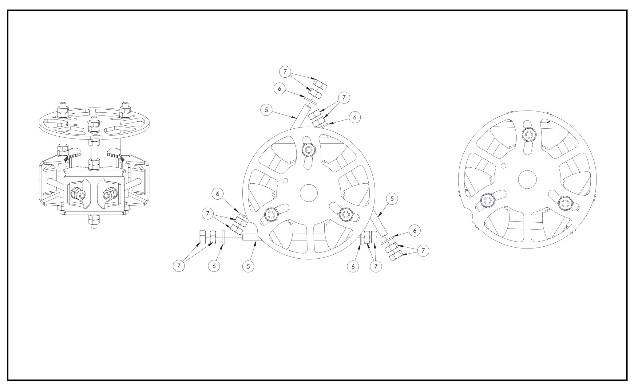
Assemble studs to pipe clamp brackets
