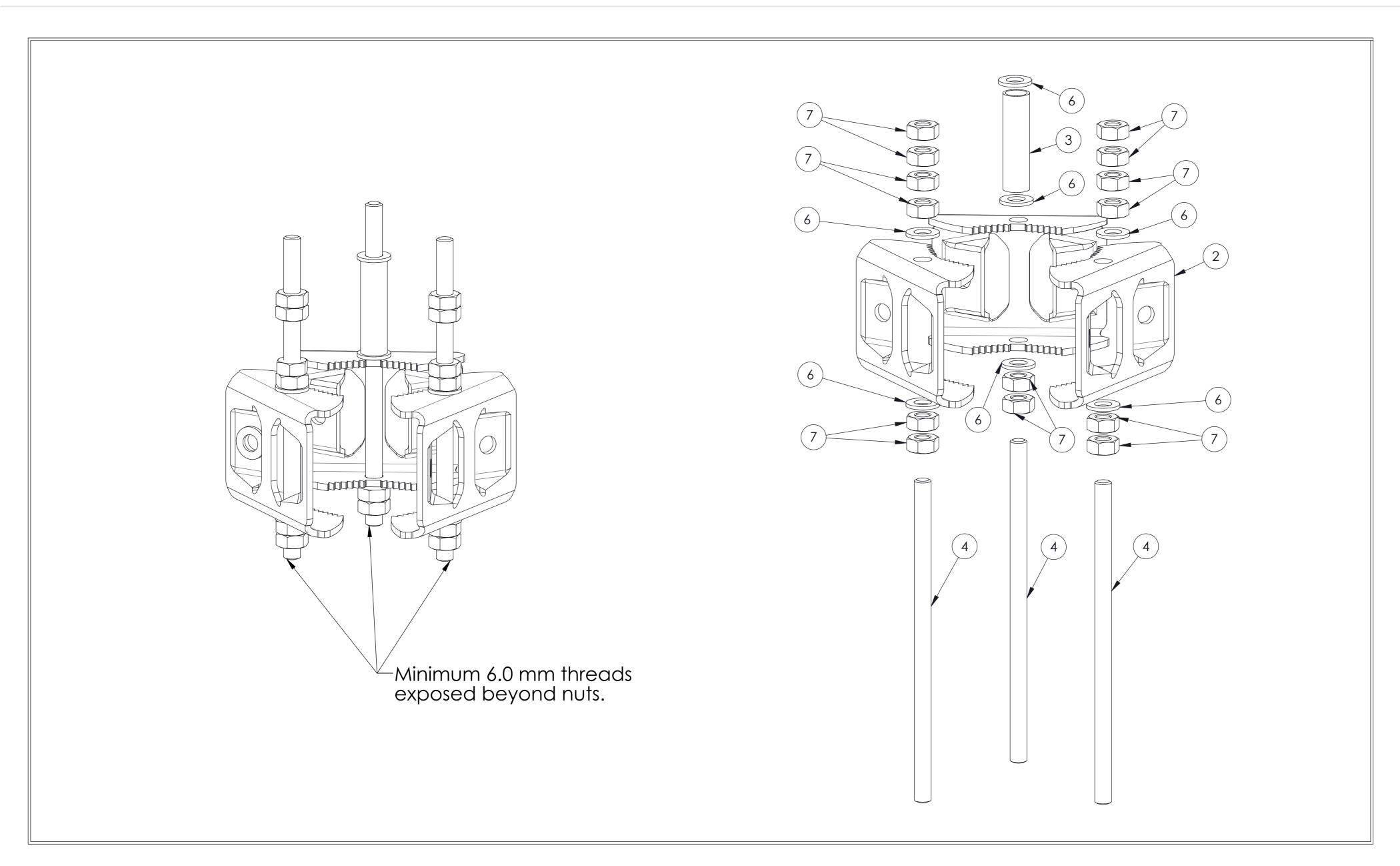
Assemble hardware to pipe clamp brackets
