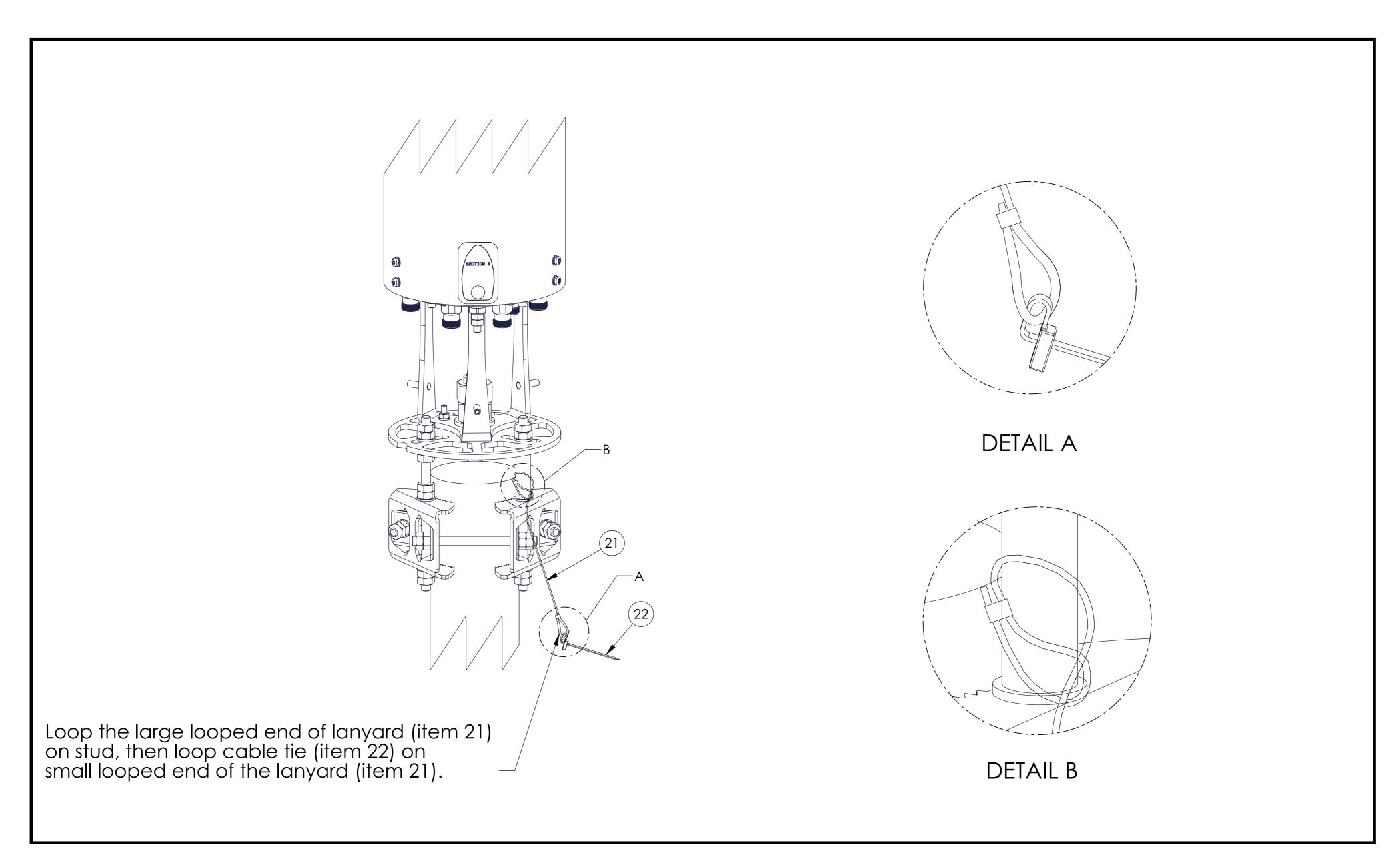
Install the lanyard on the stud
