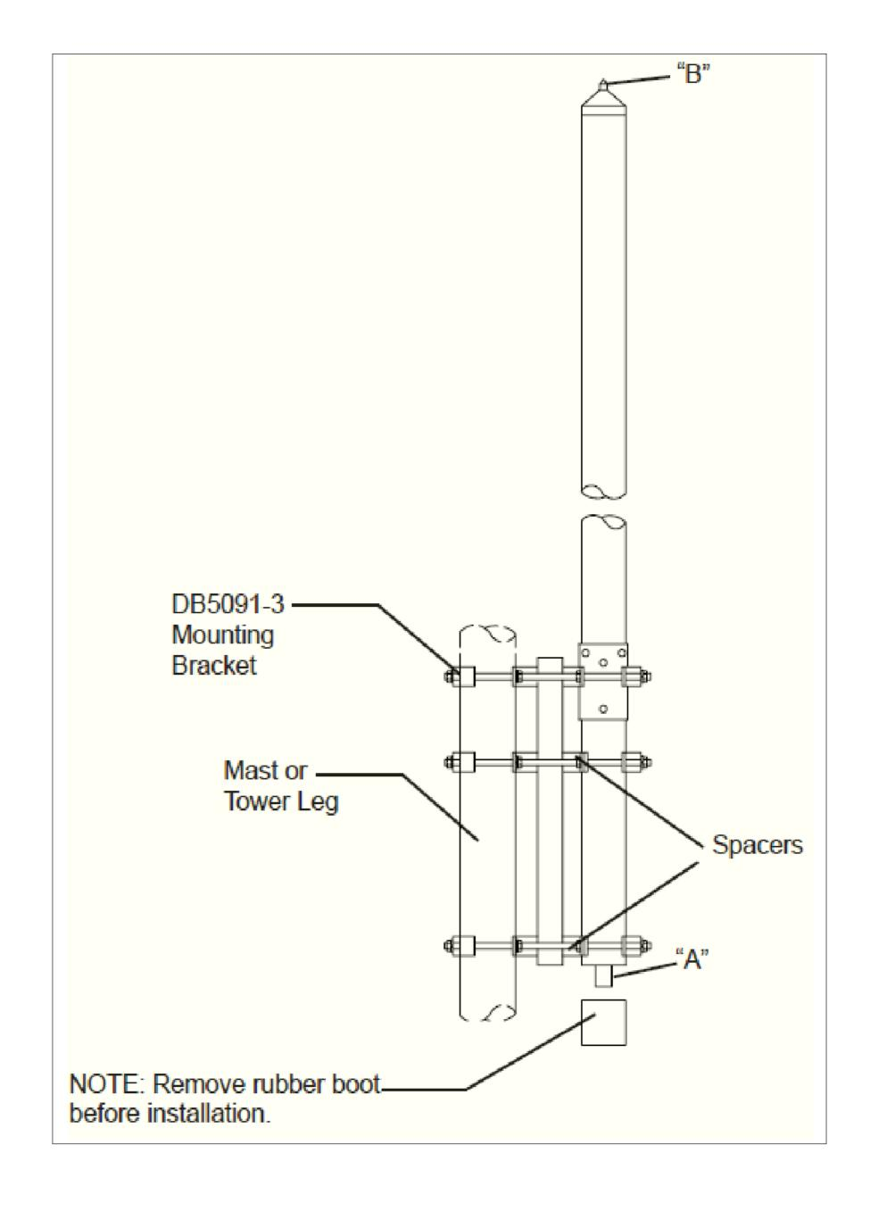
Figure 1. Antenna Using DB5091-3 Mounting Kit.
