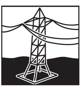
Do not install near power lines. Power lines, telephone lines, and guy wires look the same. Assume any wire or line can electrocute you.
