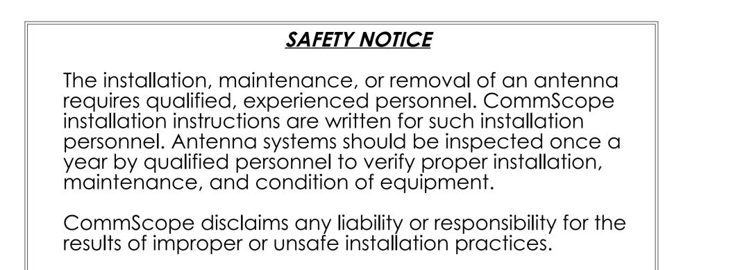
It is recommended that transmit power be turned off when the field installation is performed. Follow all applicable safety precautions as shown on this page.
