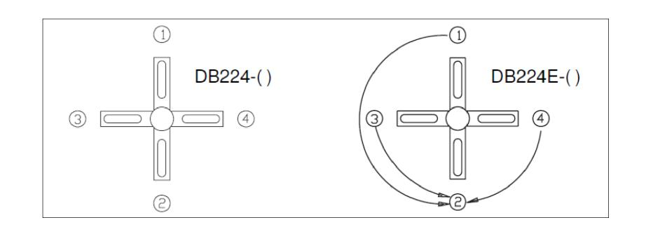
Figure 2. Top View Dipole Alignment (continued on page 2)
