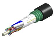
Fiber OSP cable, LightScope® ZWP Mini Single Jacket/Single Armor, 144 fiber, Gel-Filled, Stranded Loose Tube, Singlemode G.657.A2, Meters jacket marking, Black jacket color
