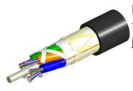
Fiber OSP cable, LightScope® ZWP All-Dielectric Self-Supporting, 96 fiber, 2.5mm Gel-filled Tubes, Singlemode G.652.D and G.657.A1, Feet jacket marking, Black jacket color
