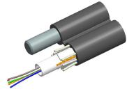
Fiber outdoor drop cable, LightScope® ZWP Self-Supporting Non-Armored Figure-8e, Singlemode G.652.D and G.657.A1, 4 fiber Arid Core construction with 0.109 in messenger, Gel-filled, central loose tube, Feet jacket marking, Black jacket color
