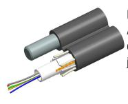
Fiber outdoor drop cable, LightScope® ZWP Self-Supporting Non-Armored Figure-8, Singlemode G.652.D and G.657.A1, 2 fiber Arid Core construction with 0.109 in messenger, Gel-filled, central loose tube, Feet jacket marking, Black jacket color
