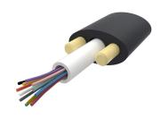
Fiber outdoor drop cable, LightScope® ZWP Self-Supporting All-Dielectric, Singlemode G.652.D and G.657.Al, 12 fiber Arid Core construction, Gel-filled, central loose tube, Meter jacket marking, Black jacket color
