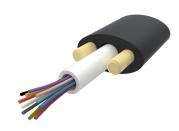
Fiber outdoor drop cable, LightScope® ZWP Self-Supporting All-Dielectric, Singlemode G.652.D and G.657.Al, 12 fiber Arid Core construction, Gel-filled, central loose tube, Feet jacket marking, Black jacket color
