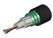
Fiber drop cable, LightScope® ZWP Single Jacket Single Armor Outdoor Drop Cable, 10 fiber Arid Core construction, central loose tube, Gel-filled, Singlemode G.652.D and G.657.A1, Meter jacket marking, Black jacket color
