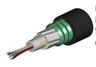
Fiber drop cable, LightScope® ZWP Single Jacket Single Armor Outdoor Drop Cable, 6 fiber Arid Core construction, central loose tube, Gel-filled, Singlemode G.652.D and G.657.Al, Meter jacket marking, Black jacket color
