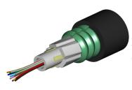
Fiber drop cable, LightScope® ZWP Single Jacket Single Armor Outdoor Drop Cable, 2 fiber Arid Core construction, central loose tube, Gel-filled, Singlemode G.652.D and G.657.Al, Meter jacket marking, Black jacket color
