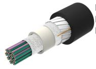
Fiber OSP cable, Non-Armored, All-Dielectric, Arid-Core, Dry Central Tube Rollable Ribbon, 144 fiber, Singlemode G.652.D and G.657.A1, Gel-free, Feet jacket marking, Black jacket color
