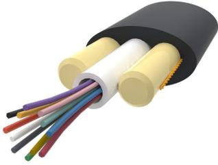
Fiber drop cable, Self-Supporting All-Dielectric, 4 fiber Arid Core construction, central loose tube, Gel-filled, Singlemode G.657.A2/B2, Meter jacket marking, Black jacket color
