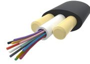
Fiber outdoor drop cable, LightScope® ZWP Self-Supporting All-Dielectric, Singlemode G.652.D and G.657.A1, 4 fiber Arid Core construction, Gel-filled, central loose tube, no ripcords, Feet jacket marking, Black jacket color
