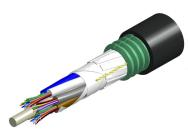
Fiber OSP cable, TeraSPEED® Mini Single Jacket/Single Armor, 48 fiber, Gel-Filled, Stranded Loose Tube, Singlemode G.652.D and G.657.A1, Meters jacket marking, Black jacket color
