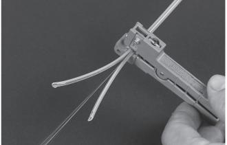
2.7 Mark the transportation tube(s) 15 mm from the tray edge (to the inside). Carefully remove the tube overlength from the mark (longitudinal slits first, then circumferential).
