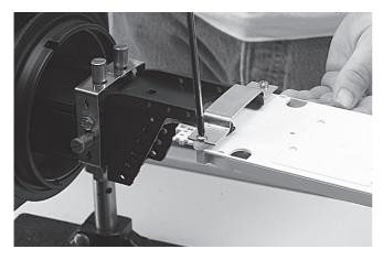
2.1 The first tray is secured against the tray tower. When necessary, replace the appropriate tray by the splitter tray.
