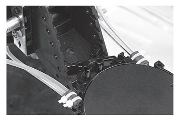
2.3 The tray can be inserted in the tray tower by aligning the tray pins (on the tray legs) with holes in the tray tower. Squeeze the tray legs and slip the tray into the tray tower.
