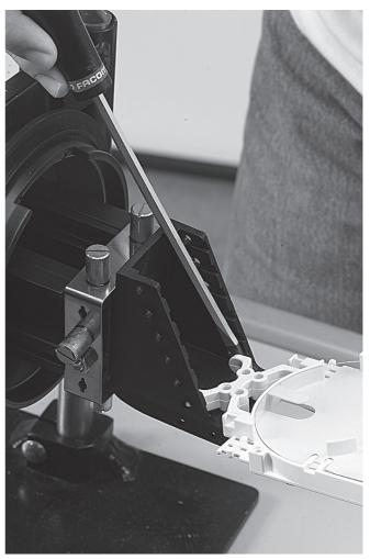
2.2 Use a screwdriver to bend one of the legs and remove the tray out of the tower.
