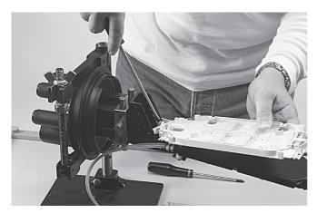
2.5 Install a splicing tray in the second slot.
