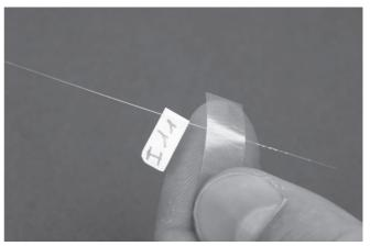
3.1 At the end of each fiber, a flag can be attached with the identification of the fiber.
