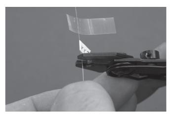
3.2 Select the appropriate fiber to be spliced, cut the identification flag when available and do all necessary steps till the splice protector is installed.
