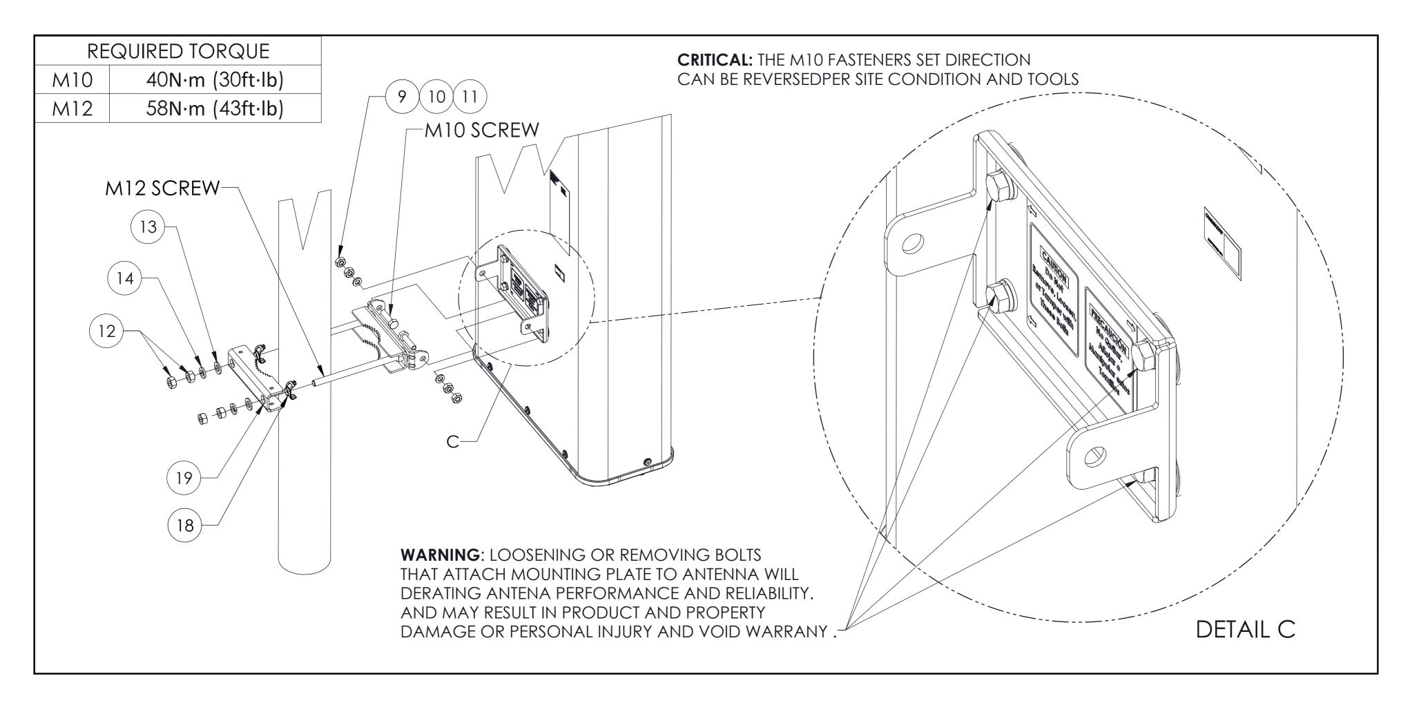
**BOTTOM MOUNT INSTALLATION** TOP & MIDDLE MOUNT INSTALLATION SAME AS BOTTOM FOR BSAMNT-4-F3
