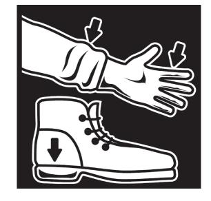
WEAR SHOES WITH RUBBER SOLES AND HEELS. WEAR PROTECTIVE CLOTHINGINCLUDING A LONG-SLEEVED SHIRT AND RUBBER GLOVES.
