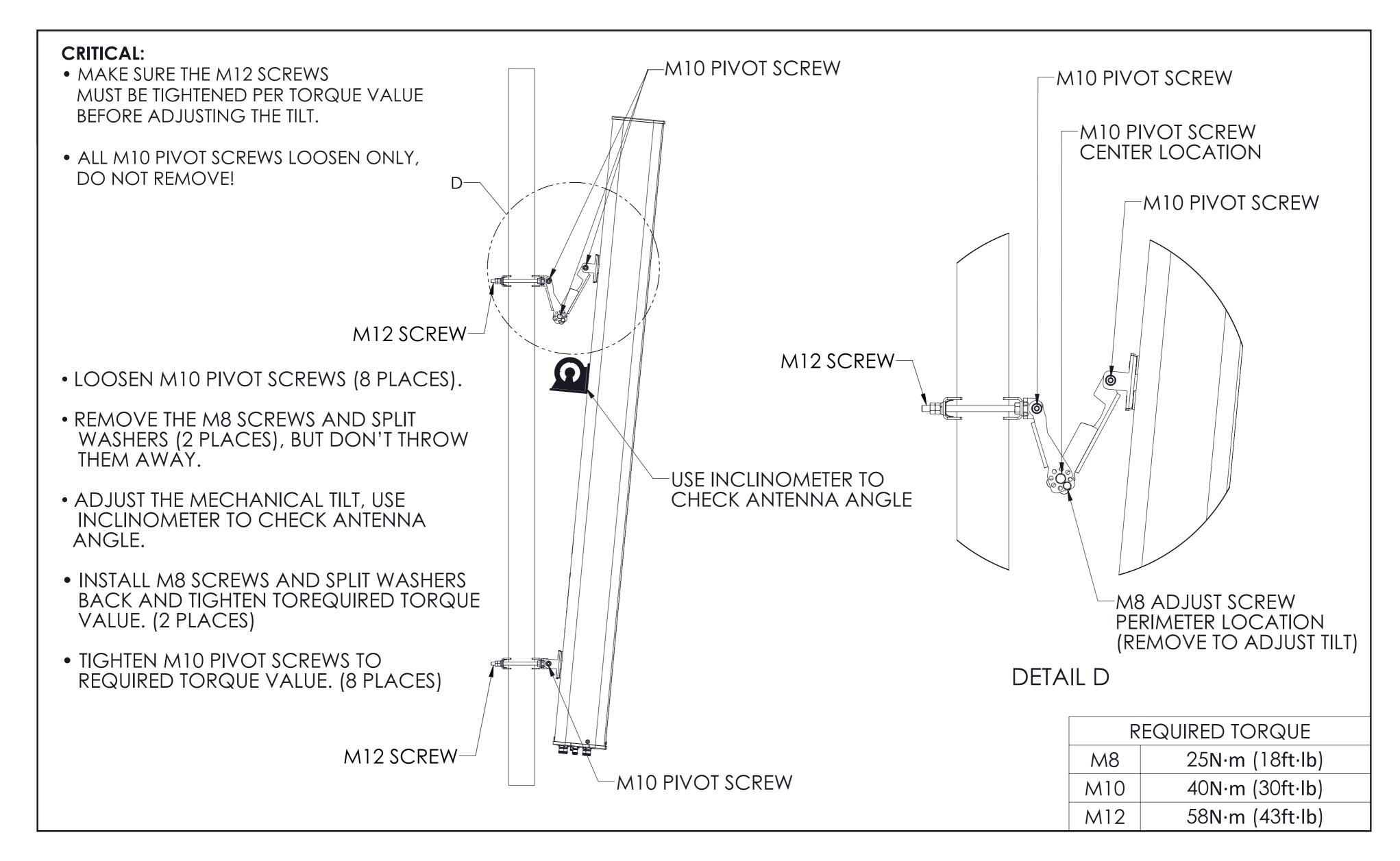
**ADJUSTING ANTENNA TILT - 2 POINT MOUNT**
