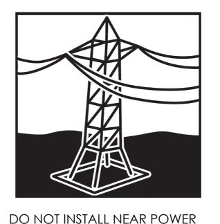
LINES. POWER LINES, TELEPHONE LINES, AND GUY WIRES LOOK THE SAME. ASSUME ANY WIRE OR LINE CAN ELECTROCUTE YOU.
