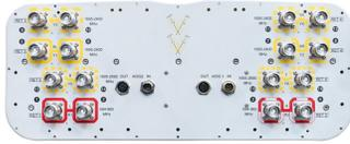
16-port sector antenna, 4x 694–960, 4x 1695–2690 MHz 65° HPBW and 8x 1695–2400 MHz 2x 2-beam 33° HPBW, 6x RET. Bands cascaded SRET
