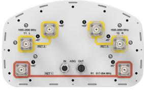
6-port sector antenna, 2x 617-894 and 4x 1695–2690 MHz, 65° HPBW, 3x RET, 600 MHz-Ready Antenna Technology
