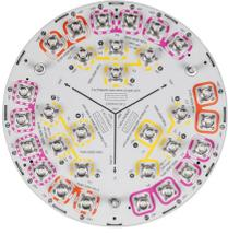
30-port small cell antenna, 12x 1695–2690, 12x 3400–3800 and 6x 5150–5925 MHz. 360° Horizontal Beamwidth, fixed tilt.
