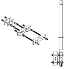
Fixed Tilt Pipe Mounting Kit for 2.0"-4.5" (50-115mm) OD round members for omni antennas. Includes 2 clamp sets.
