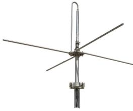
1-port omni ground plane antenna, 450–470 MHz, 360° HPBW, fixed electrical tilt. Bandwidth: 2% of frequency.
