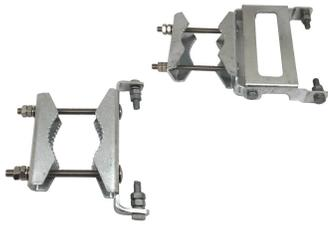
Wide Profile Antenna Downtilt Mounting Kit for 2.4 - 2.8 in (60 - 70 mm) OD round members. Kit contains one tilt top bracket set and one bottom bracket set.
