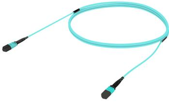
OM4 MPO12 (Pinned) to MPO12 (Unpinned), Fiber Trunk Cable Assembly, 12-Fiber, Method A, Low Smoke Zero Halogen
